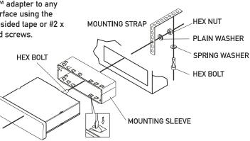
TYPICAL FRONT-LOAD DIN MOUNTING METHOD
